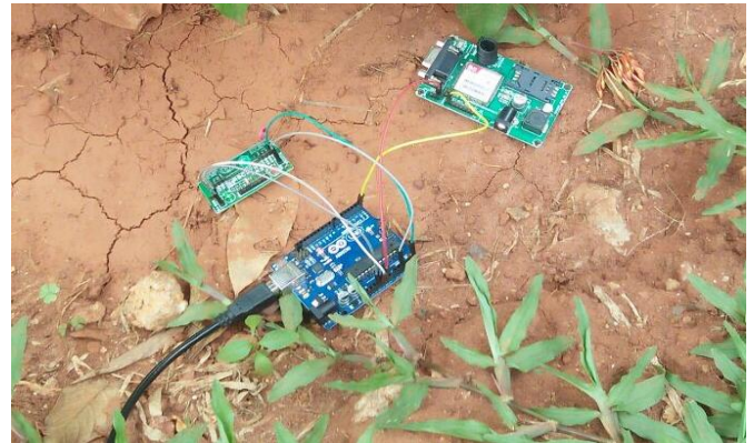
Fig.3 Receiver section of the proposed system
