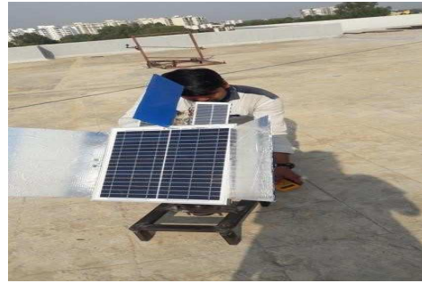
Figure 3: Sun Tracking with Reflectors
